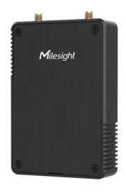
UG56 is a robust 8-channel indoor LoRaWAN® gateway. Adopting SX1302 chip and high-performance quad-core CPU, UG56 supports connection with more than 2000 nodes. UG56 has line of sight up to 15 km and can cover about 2 km in urbanized environment, which is ideally suited to smart building, smart industries and many other indoor applications.
